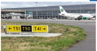
Signs are one of the biggest equipment near the runway. Signs may collapse or be damaged due to jet blast, collisions with vehicles or extreme winds.
